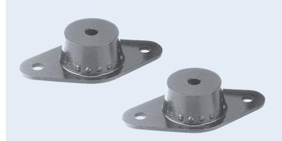
Barry HR Series mounts are best suited for isolation of diesel engines with five or less cylinders for on or off-highway applications. The standard neoprene elastomer provides resistance to oils and most solvents. Other elastomers are available, consult factory for more information.
